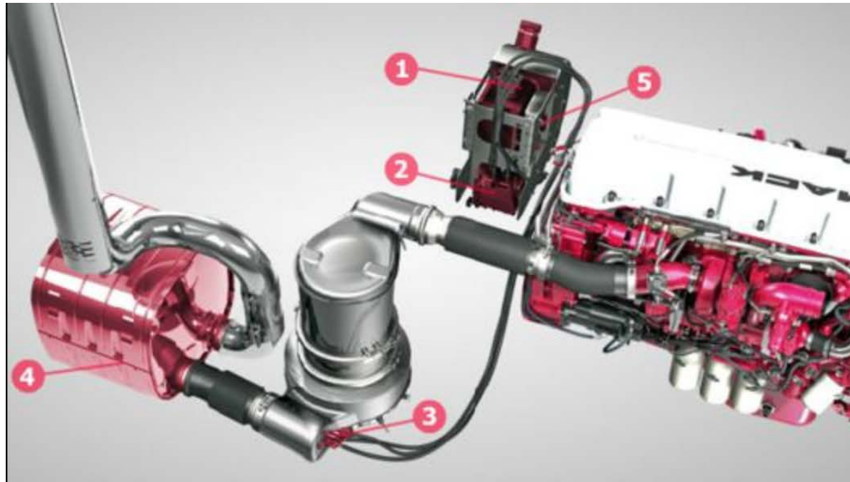
Figure 13. SCR System on US 2010 Mack MP7 Truck Engine
